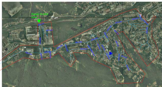
Selected District Metering Area (DMA) in Tuzla
