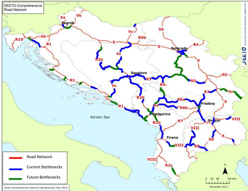
Figure 9. Identified Current and Future Bottlenecks on the Existing SEETO Comprehensive Road Network for the Low/Moderate Economic Growth Scenario
