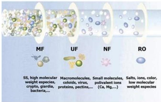
**Figure 12.4:** Ultrafiltration (UF) processes utilize a semi-permeable membrane to separate microcontaminants from a water stream.
