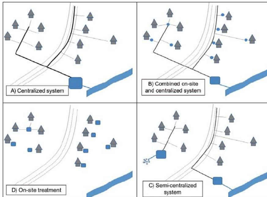
**Figure 12.1:** Different wastewater treatment systems
